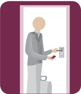
Enter room: Lock checks that keycard has correct information (room #, unique hotel code, time window etc.).
