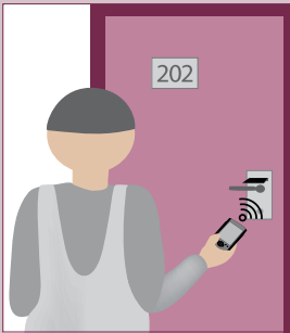
Locklink/program lock: Upload software and data to lock (room #, unique hotel code, set clock).
